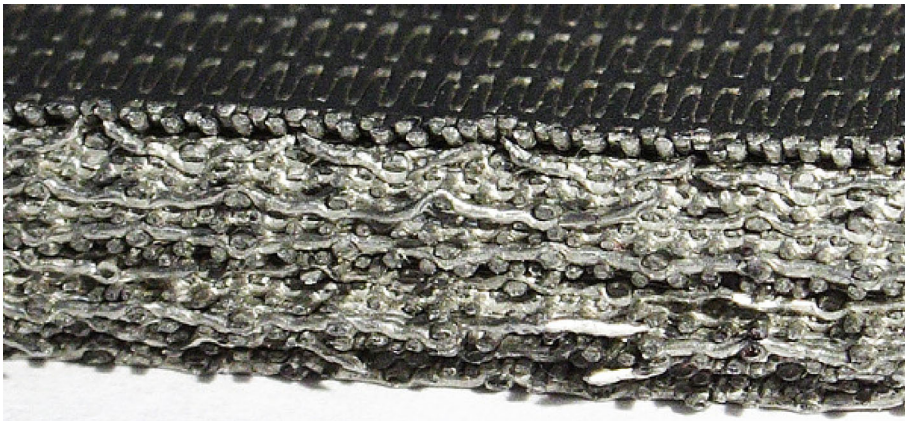
Figure 2. Rigimesh cross-section after bending fracture
